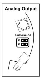
Figure 16: EFM-100C jumper configuration
