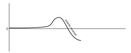
Figure 35: Electric Field Polarity Reversal
