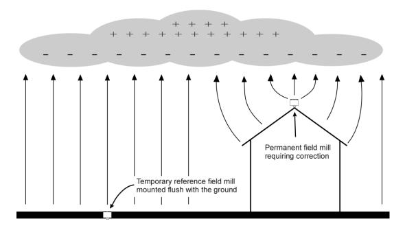
Figure 18: Correcting a Field Mill using a Reference Field Mill
