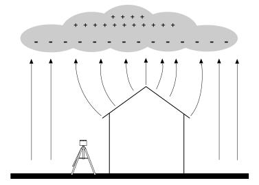
Figure 6: A poor choice of mounting locations
