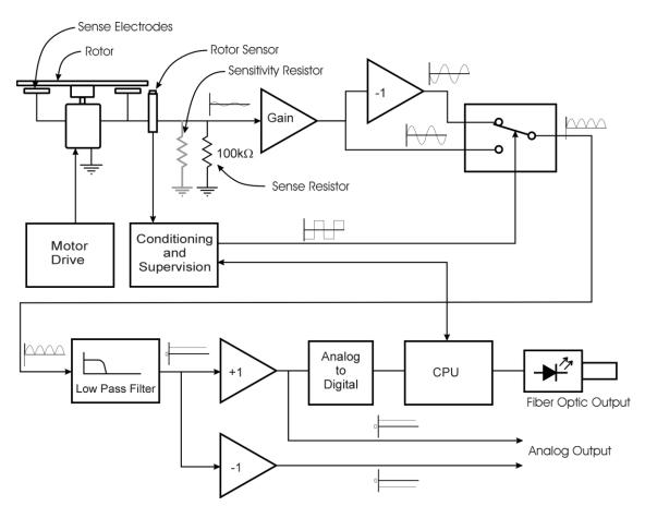
Figure 3: Field Mill Block Diagram
