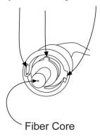
Figure 14: Male Fiber Optic Connector
