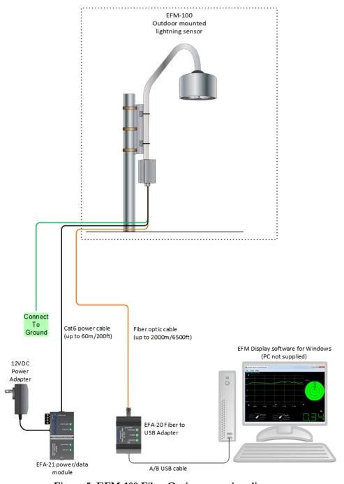
Figure 5: EFM-100 Fiber Optic connection diagram
