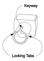
Figure 13: Female Fiber Optic Connector
