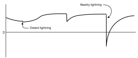
Figure 38: Step Changes in Field Magnitude Indicate Lightning
