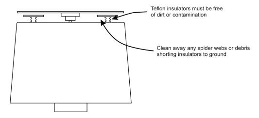
Figure 40: Field Mill Cleaning
