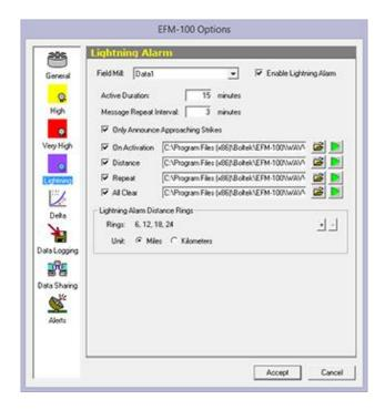
Figure 23: EFM Options – Lightning Alarm
