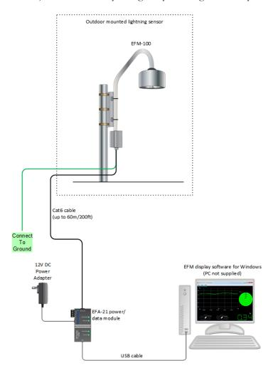
Figure 4: EFM-100 Standard Connection Diagram
