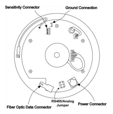
Figure 15: EFM-100C Field Mill Connections
