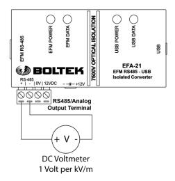
Figure 9: EFA-21 Voltmeter Connections – Differential (Preferred Connection)
