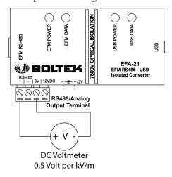
Figure 10: EFA-21 Voltmeter Connections – Single Ended
