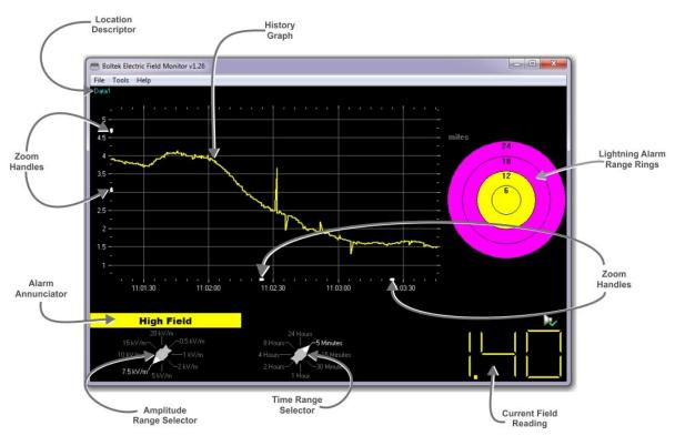
Figure 31: EFM-100 Software Display
