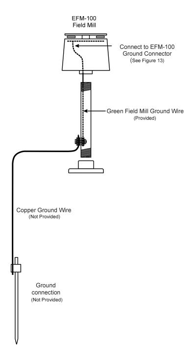
Figure 19: Field Mill Grounding Detail
