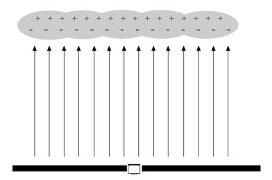
Figure 1: Electric Field Mill at Ground Level
