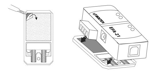
To attach the clip to a DIN rail, first slide the end with the spring into the rail, then push up and in towards the back, then release to lock in place as shown in the diagram below.
