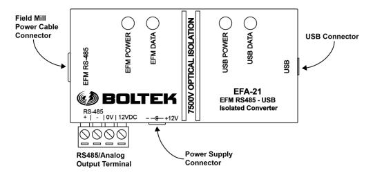
Figure 8: EFA-21 Power/Data Module Connectors
