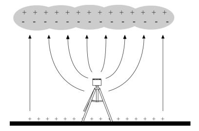
Figure 2: Intensification of Electric Field
