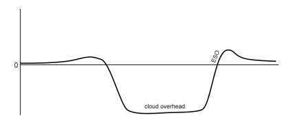
Figure 37: End of Storm Oscillation
